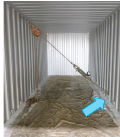
Lashing Ring (Bottom side rails) Max pull test 2250kg, 10x2
