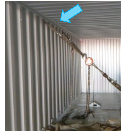
Lashing Ring (Top side rails) Max pull test 2250kg, 10x2
